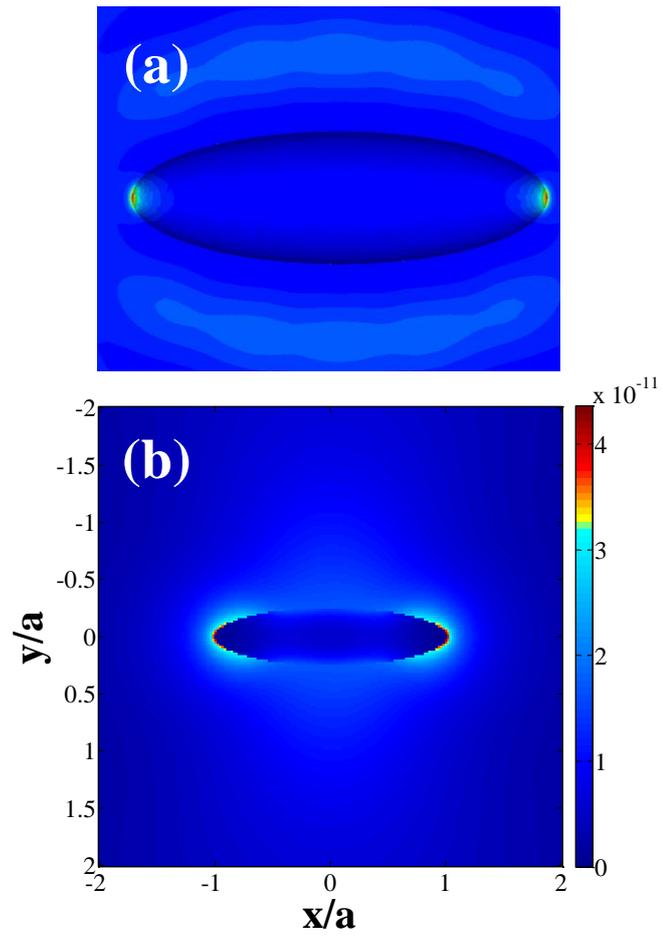
**Figure 7.** Electric energy distribution  $[J / m^3]$  in  $z=0$  plane, as generated by both method. (a) CST (b) SMT.
