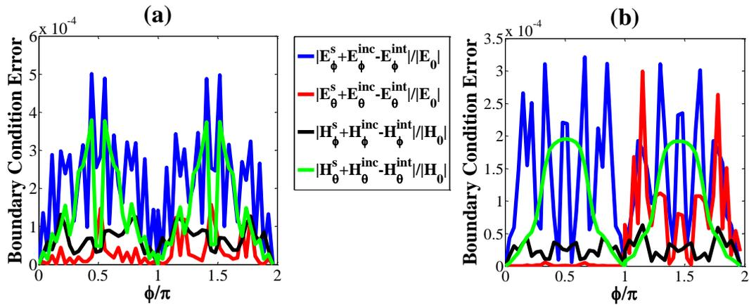
**Figure 4. Boundary Condition Error in the continuity of tangential electromagnetic components, for BEM and SMT. The error was calculated in  $Z=0$  plane along the longest contour. (a) BEM (b) SMT & SCBSD**
