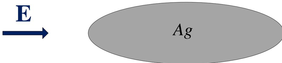
**Figure 3. Plane wave excitation of a silver spheroid. The electric field is polarized along the major axis.**
