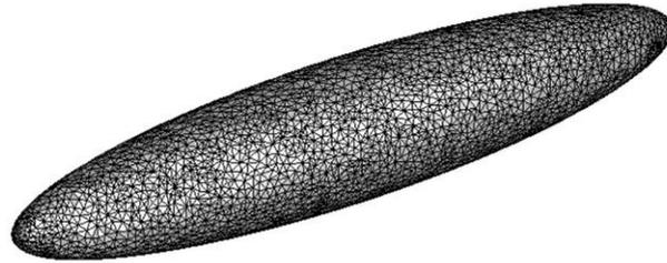
**Figure 5. CST parameterization of ellipsoid. Areas of small radii of curvature are refined.**
